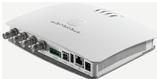
Figure 7.5: The passive RFID antenna router that we have used in our experiments [31].
